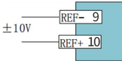
Figure 4.3.2 Analog input wiring of external power supply
