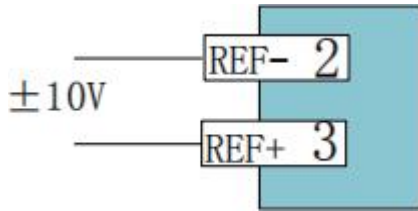
Figure 4.3.2 Analog input wiring of external power supply
